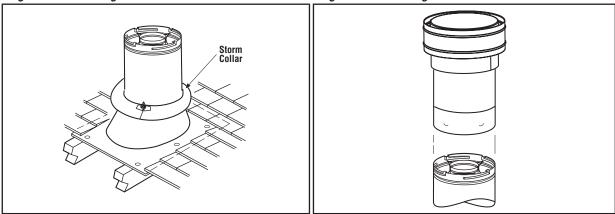
**13. Install the vertical termination**—Extend the vent sections to the correct height (*Figure 3*). The SV4.5CGV-1 Vertical Termination (*Figure 21*) installs in the exact same fashion as any other Secure Vent<sup>®</sup> section.
