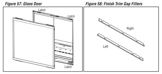
**3.** Carefully grip the door at the top and bottom, and align it with the fireplace opening. Lightly press against the door, to hold it in position.
