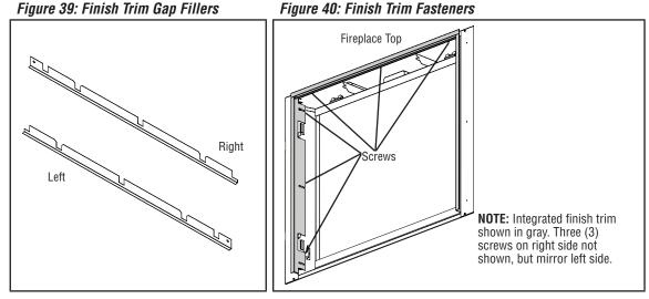
**4.** Loosen the nine (9) screws securing the integrated finish trim and slide the trim out and away from the fireplace door (*Figure 39*).
