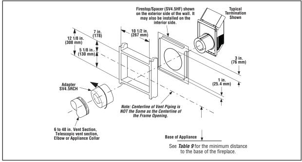
Figure 25: Installing the Horizontal Termination
