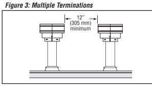
Terminate single vent caps relative to building components according to Table 5 and Figure 3.
