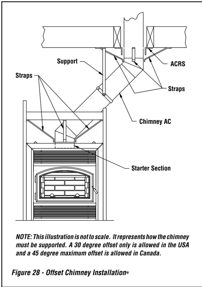
Figure 28 - Offset Chimney Installation\*
