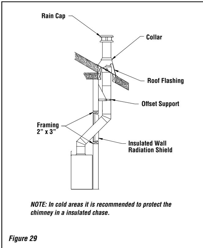
NOTE: In cold areas it is recommended to protect the chimney in a insulated chase.
