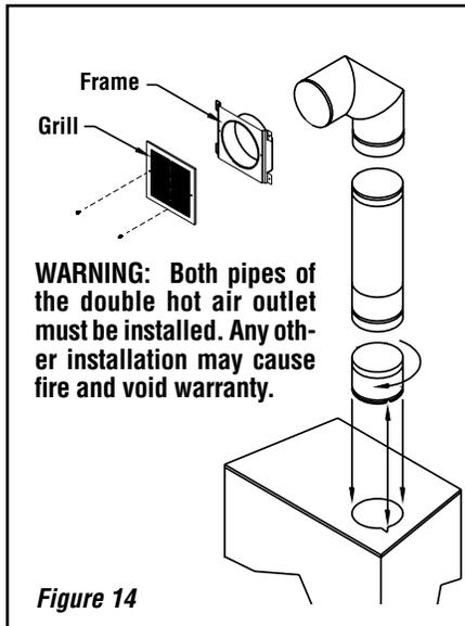
For safe installation, the gravity kit must meet the following requirements:
