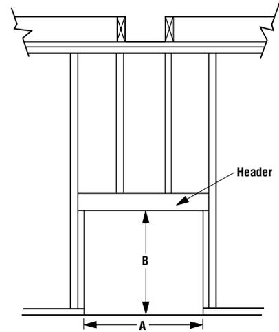
Combustible materials can NOT be used in the space directly above the fireplace. Do not fill the space above the fireplace with any material (Except the wood framing)
