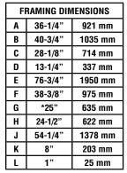
Total depth is 25-1/2 inches including the back spacer minus 1/2 inch for drywall to be flush with the facing.
